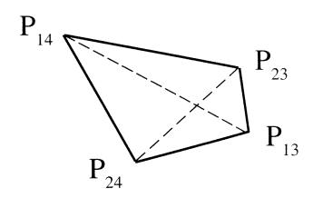
If this is an *Opposite Pole Pair Quadrilateral* then, by definition, the *diagonals* are the lines from  $P_{14}$  to  $P_{23}$  and from  $P_{24}$  to  $P_{13}$ .
