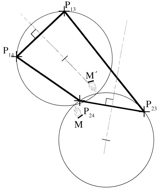
The have just succeeded in constructing—count 'em— not one but two centerpoints, M and M'. The places where the two circles intersect see opposite sides of the opposite pole pair quadrilateral under equal angles! Call out the brass band! (Actually, the angles may not be equal but may differ by 180° from one another, but they still satisfy the requirements for valid centerpoints.)
