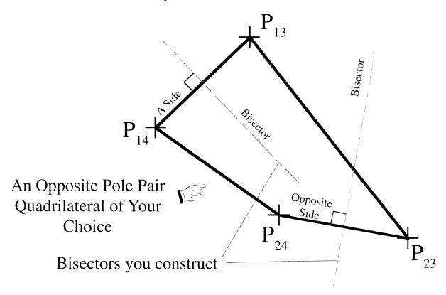
From the pole at the end of one of the sides lay out an arbitrary signed angle  $\alpha$  as shown on the next figure. Mark the point where it cuts the bisector to that side. (Since I laid out the angle on the side with a #1 subscript in common, I am labeling this point  $B_1$  so as not to get confused.) (B as in "Bisector" and 1 as in "1", get it?)
