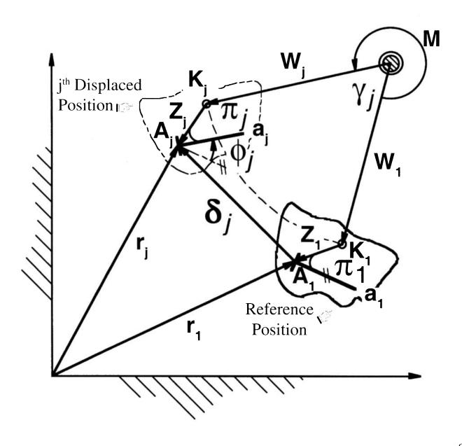
In the reference position, the unknown circlepoint,  $K_1$  bears a certain unknown relationship to the known point  $A_1$ . Let the unknown vector  $\mathbf{Z}_1$ , <u>rigidly attached to the moving plane</u>, locate point  $A_1$  with respect to  $K_1$ .
