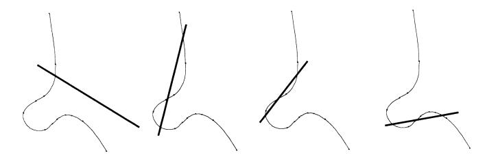
Even though the curves usually look like octopi, they often break off like a droplet and have two branches as in this case. The straight line rule still works, as this is just a single cubic curve even though it has two parts.
